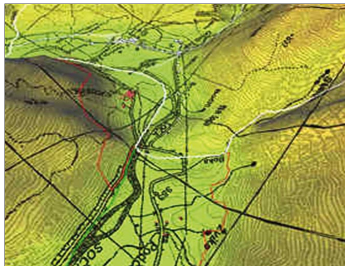
Figure 2. A typical complex map tile, with elevation, map and vector data
